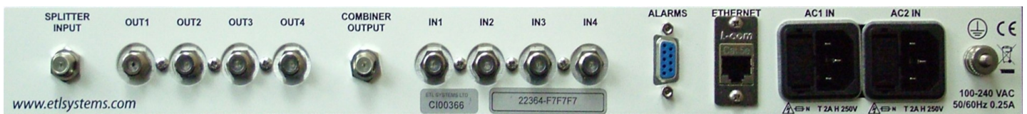
Rear View of Model 22364-F7F7 (Supplied with 75 ohm F-type connectors)
